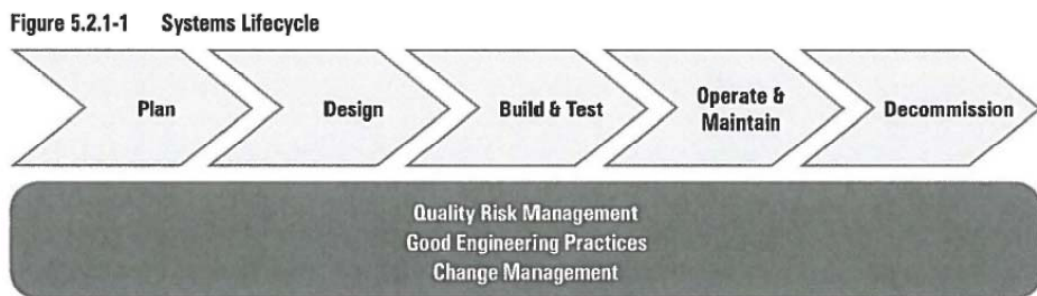
Figure 5.2.1-1 Systems Lifecycle图5.2.1-1系统生命周期
